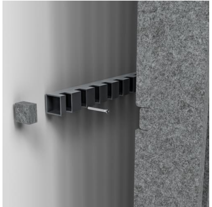
Baffle Systems Direct Mounting Detail
