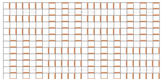
Mesh Baffles Checkered Configuration
